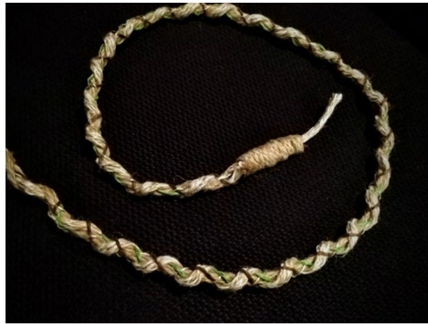
Above: Some work-in-progress photos of me braiding the rope sensors using a combination of coloured twine, rope string and LED string lights. Three different connections are outputted from each rope sensor (the touch sensor, power and ground for the lights).
